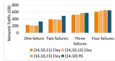
Figure 16: Average network traffic evaluation of C4-C6 against RS codes ( W_1 workload, multiple-PG).
